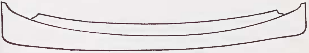
Fig. 6. Addition of wash-strakes in the midbody.
